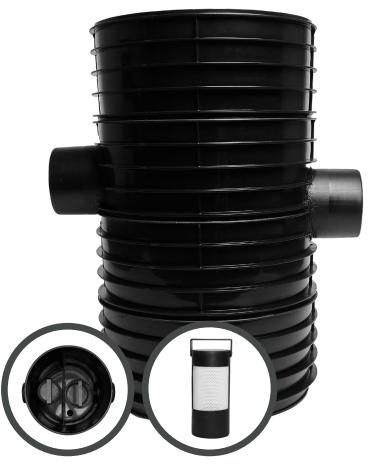
The HydroCell450 Advanced is located up stream of large sized attenuation, retention and infiltration systems. This model comes with a double filter system which is designed to separate debris and any unwanted particles before entering and blocking the downstream pipework. The HydroCell450 Advanced improves the quality of water before it is reintroduced back into the drainage system.
