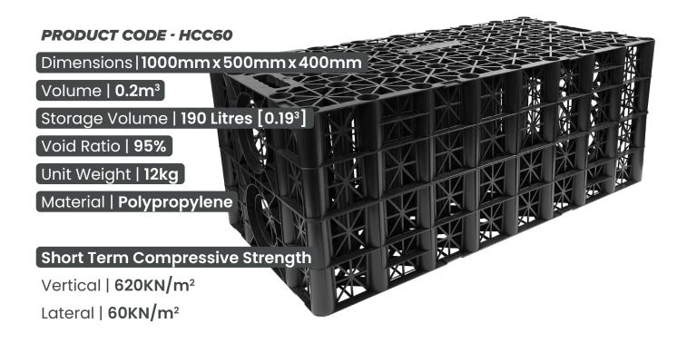
HydroCell crates are designed for highload applications at greater depths, making them suitable for residential, industrial, and civil engineering projects. They offer a compressive strength of 62 tonnes/m<sup>2</sup>.
